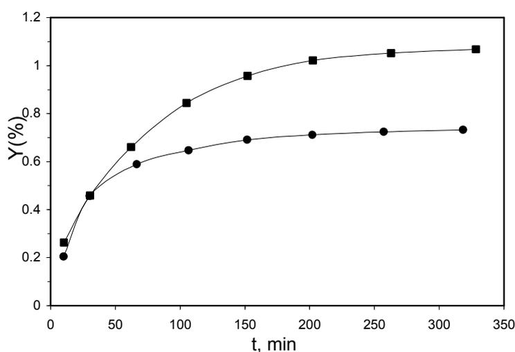
**Figure 1:** Yield of extracted volatile oil from coriander at mean particle size 0.6 mm. ■ -150 bar and 40°C; ● - 90 bar and 40° C.
