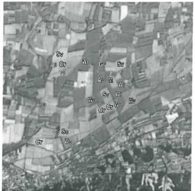
Figure 1: 5 km x 5 km SPOT-XS image acquired on March 25, 1997 over the Alpilles-ReSeDA site, along with ground-truth fields; M: meteorological site; W: wheat; S: sunflower; A: alfalfa; C: corn; G: grass; c: calibration fields; v: validation fields; r: remote sensing fields.
