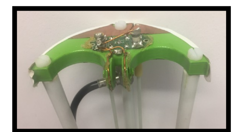
Helmholtz coil designed for the fruit pedicel
