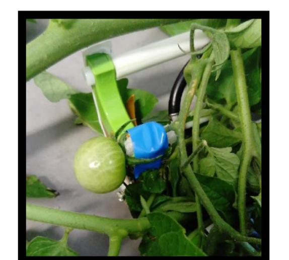
Helmholtz coil designed for the fruit pedicel
