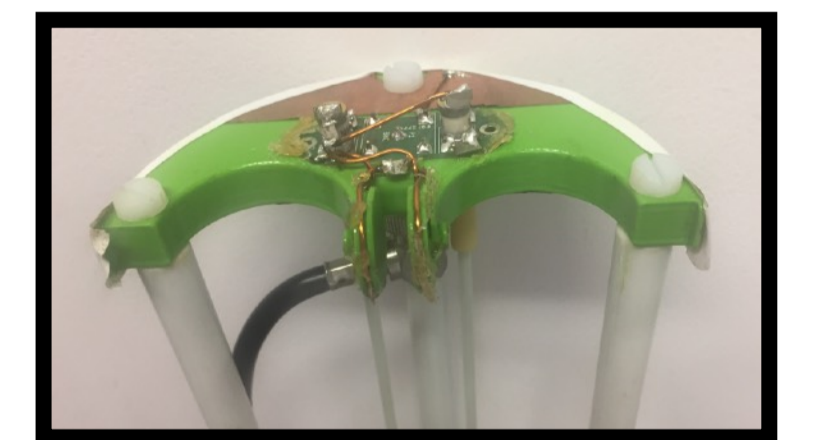
Helmholtz coil designed for the fruit pedicel
