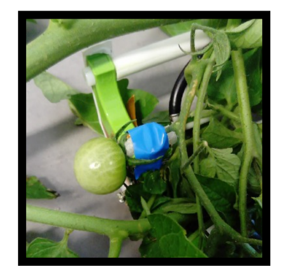
Helmholtz coil designed for the fruit pedicel
