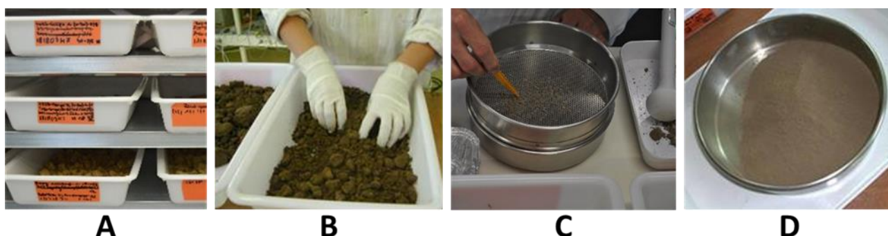
Figure 12. Sample preparation. A) drying the sample; B) loosening the sample; C) remove stones and roots; D) fine earth.
