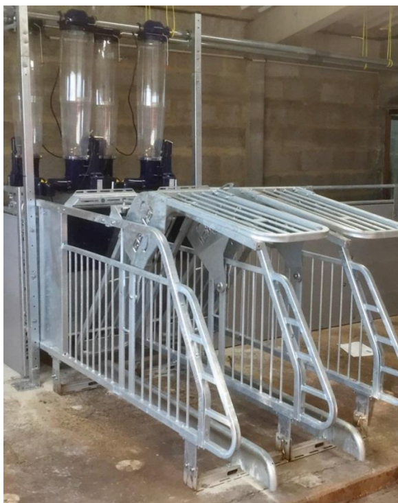
Photo 6. Feeding stalls for gestating sows. The feeding stall operates mechanically. The sow enters the feeding stall and the door behind her is closed.
