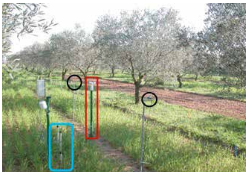
Figure 1. Photo taken in the AF treatment showing the position of two PAR (Photosynthetically active radiation) sensors (black circle), of the anemometer (red) and of the four tensiometers (blue).
