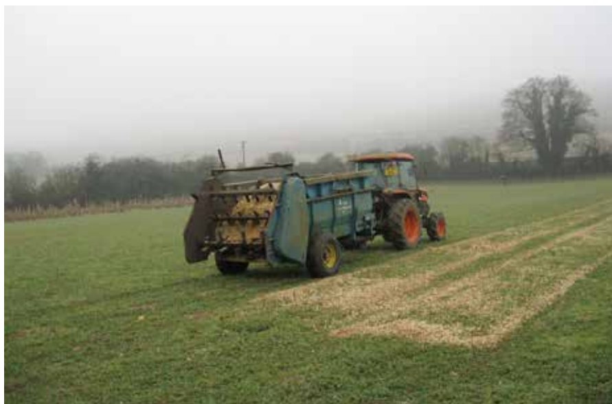
Figure 1. Spreading ramial woodchip at Tolhurst Organics using a rear discharge muck spreader, 2018
