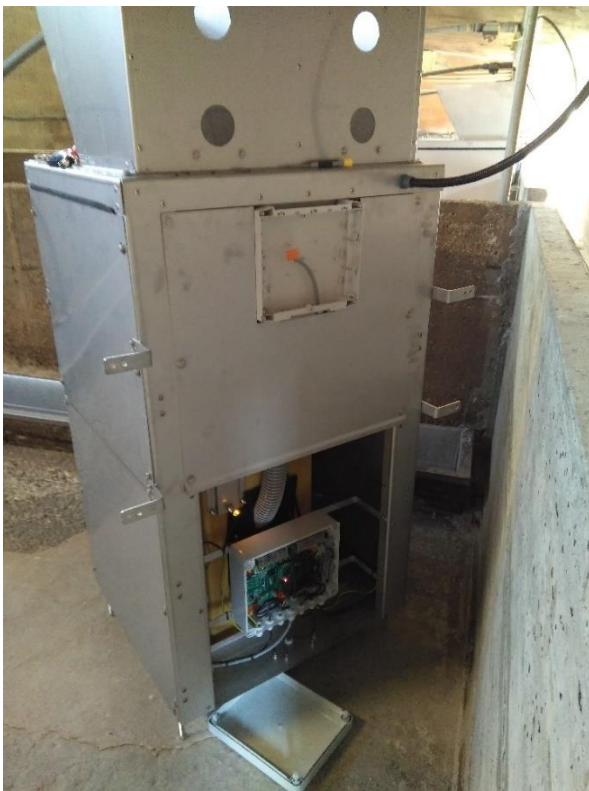
Motherboard based on a microprocessor that controls all the sensors and actuators of the feeder.
