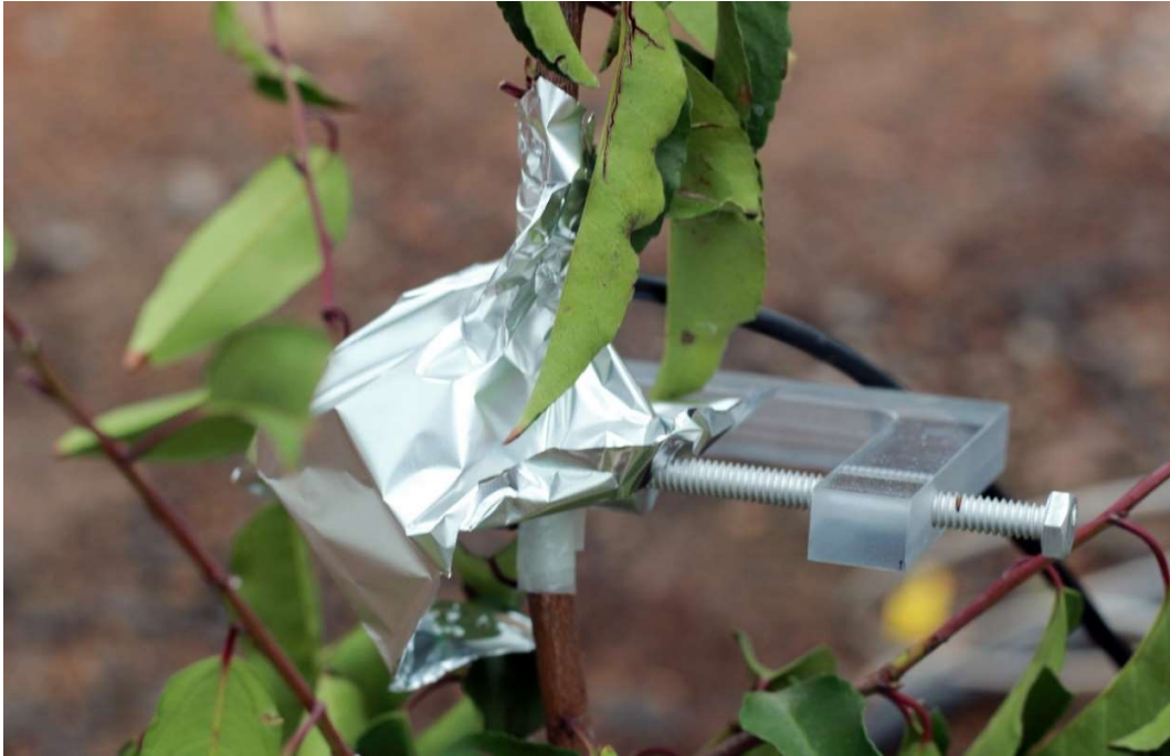
Figure 17: ICT psychrometer covered in aluminum foil to protect it from direct sunlight exposure.
