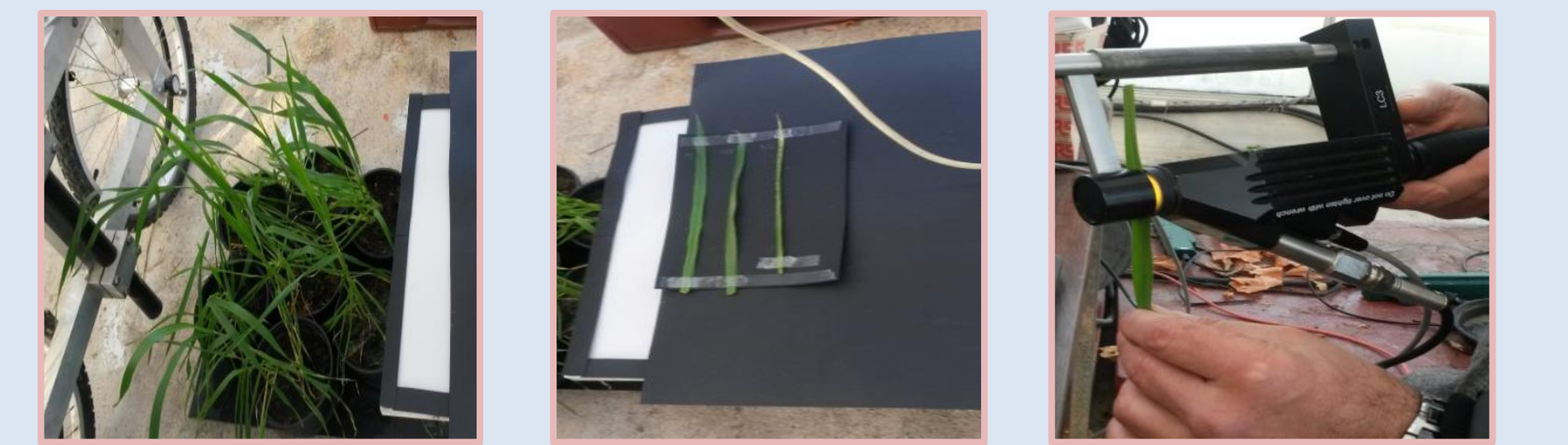
Focal pot surrounded by 6 pots, in order to reproduce as much as possible the conditions of multiple reflections. Three individual leaves removed from the focal pot and placed on black paper to be imaged without multiple reflections. Nitrogen measurement at 4 different points along each leaf, using an ASD field spectrometer reflections.
