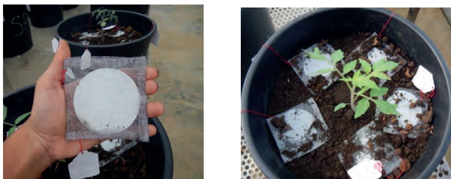
Figure 1: Litterbags (8,5 x 8,5 cm) with cellulose paper (Wattman, 7 cm) (Pictures C.Moulin).
