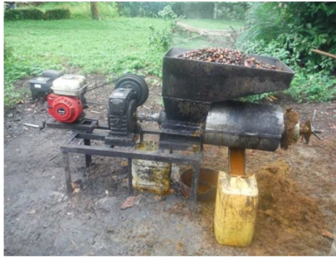
Figure 22 (D. Nanda): Continuous motorised screw press (Caltech type). This model has a mechanical speed reducer between the engine and the press. Motorised models are sold from about one thousand dollars for the cheapest to a few thousands for the best ones.
