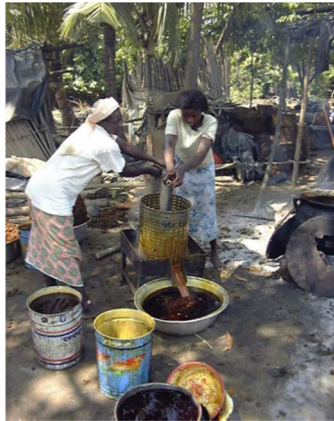
Figure 19 (S. Rafflegeau): Pressing with manual discontinuous press, a smaller model appreciated by women producers in Côte d'Ivoire because of its cheap price (few tens of dollars) and facility of handling.
