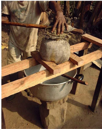
Figure 17 (S. Rafflegeau): The cooked fruits are manually mashed in the traditional mortar, and then are put in a bag and oil is extracted by pressure using a stick.
