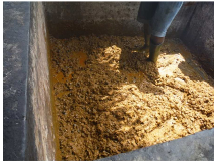
Figure 14 (D. Nanda): Traditional extraction by foot treading and washing with water inside a concrete basin.
