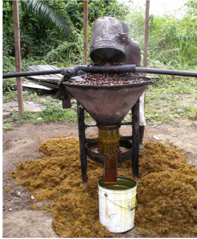
Figure 21 (S. Rafflegeau): Manual continuous screw press (Caltech type). This vertical model is sold for a few hundreds of dollars in Cameroon.
