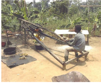
Figure 16 (S. Rafflegeau): Adaptation of a traditional cassava press for palm oil extraction.
