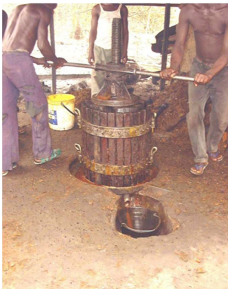
Figure 18 (S. Rafflegeau): Pressing with manual and robust discontinuous press imported from Nigeria to Southwest Cameroon for a few hundreds of dollars.
