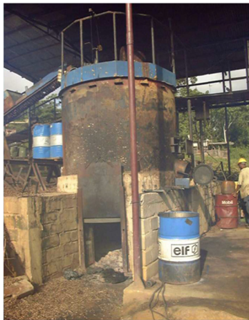
Figure 7 (S. Rafflegeau): Examples of investment in the mini-mill, a semi-industrial extraction unit, by managerial enterprises of producers: view of a self-made steam FFB cooker in Cameroon.
