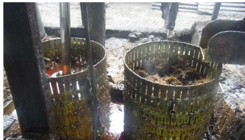
Figure 20 (D. Nanda): Hydraulic discontinuous press: the cooked fruits are mashed with a digester. The mass is placed in a heavy metal cage and a metal plunger is used to press the materials. The pressure should be increased gradually to allow time for the oil to escape. The plunger can be moved manually or by a motor. If the depth of mass is too great, oil will be trapped in the centre of the mass.
