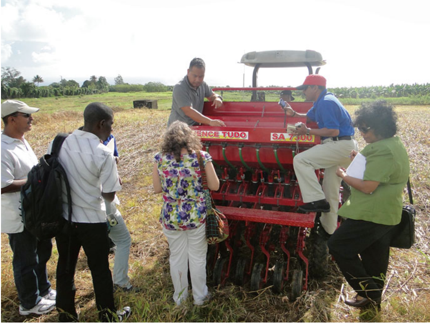
On field discussions on a seeder adapted to direct sowing in tropical wet areas. © 2013 Magalie Lesueur Jannoyer
