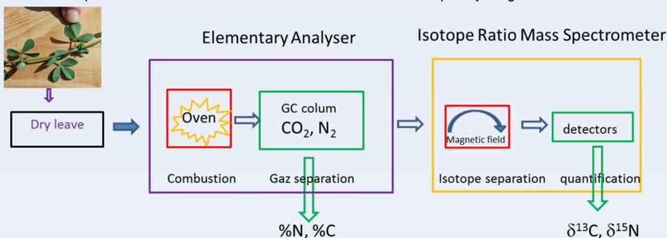
The %C, %N,  $\delta^{13}\text{C}$  and  $\delta^{15}\text{N}$  were measured on a Isoprime 100 IRMS coupled with a elemental analyser (Microcube).
