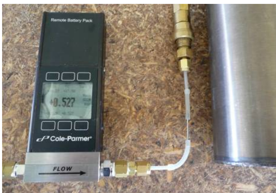
Figure 5.11: A flow meter must be on the atmospheric side of the restrictor when measuring flow.
