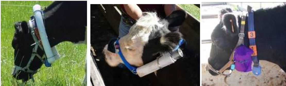
Figure 5.14: Various canister mounting positions.
