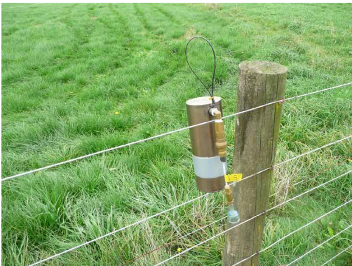
Figure 7.3: Equipment for sampling the background air can be hung on a fence.
