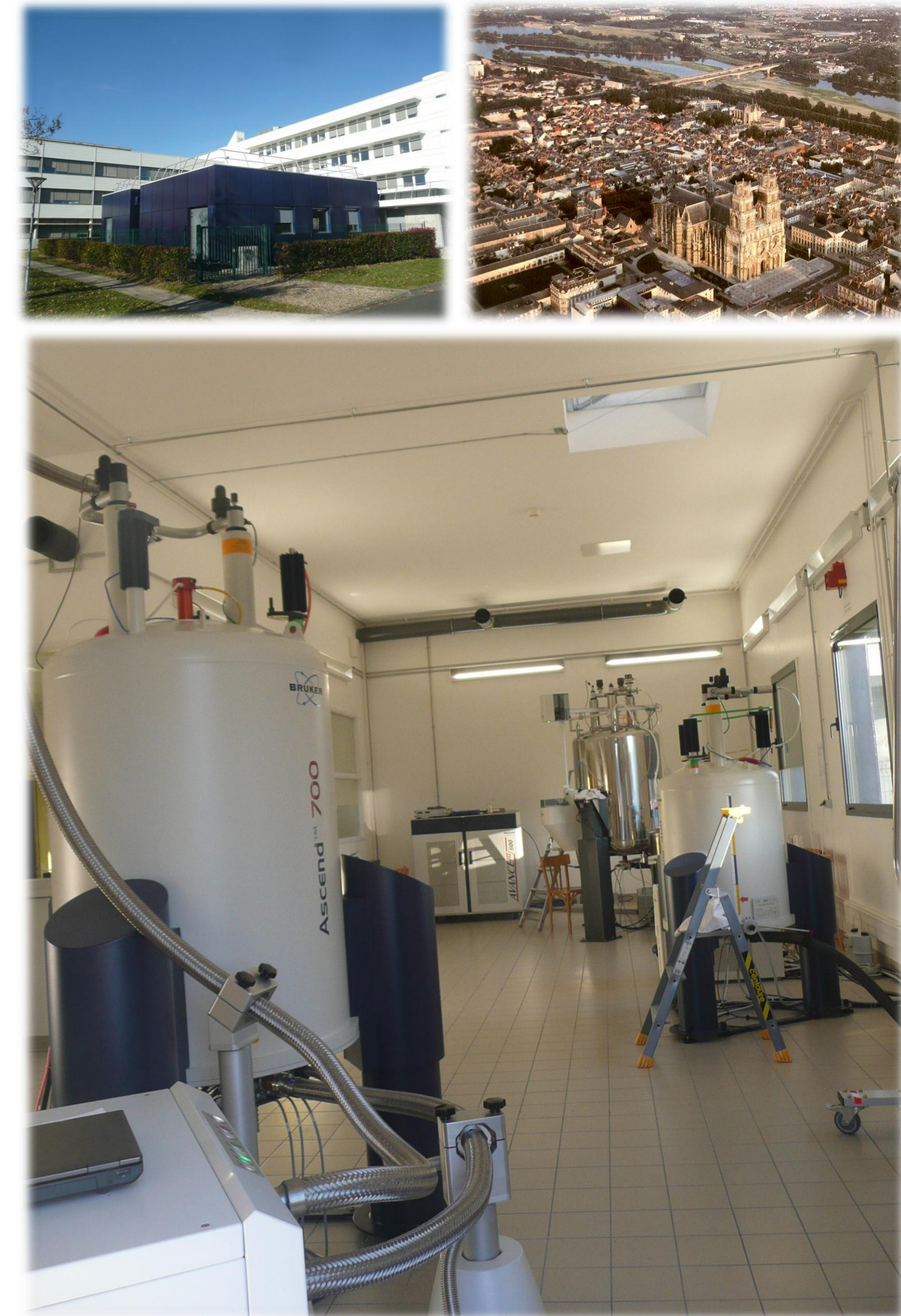
Front to back : BRUKER AVANCEIIIHD 700MHz with TCI cryoprobe, BRUKER AVANCEIIIHD 400MHz, BRUKER AVANCEIII 600MHz
