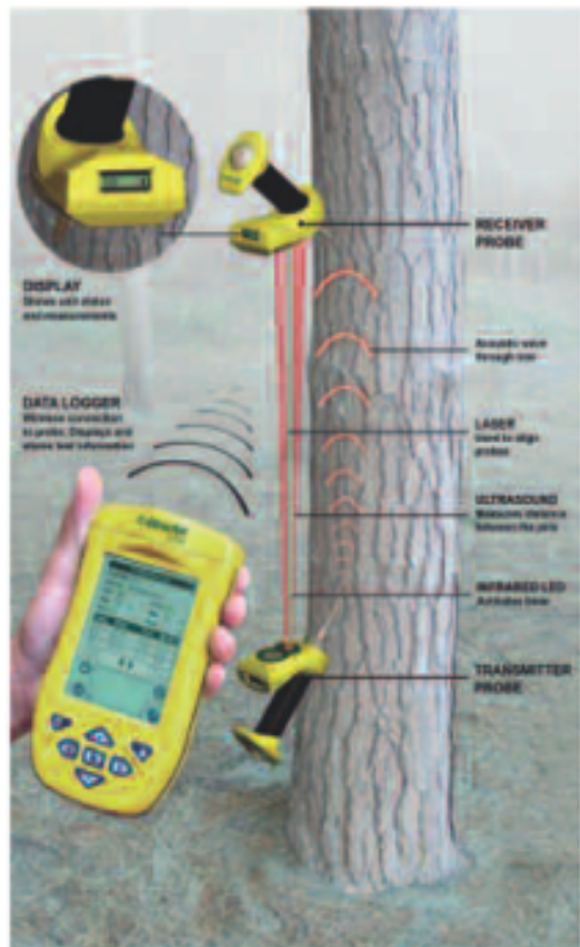
Figure 2 Portable acoustic tool for measuring stress wave velocity in standing trees using the time-of-flight method.
