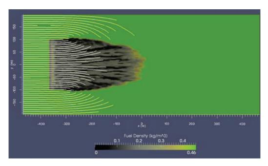
Figure 2. Top down view of 6 m s<sup>-1</sup> wind 200 m-ignition fire. This image illustrates the parabolic shape of the progressing fire and the white streamlines illustrate the interaction between the upstream air flow and the competing indrafts of the flanking and heading firelines
