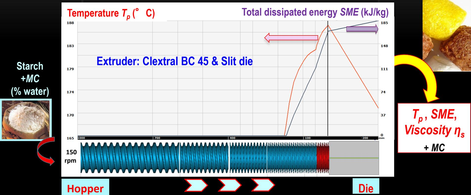
« Ludovic®'s output variables at die exit = input of expansion model »
