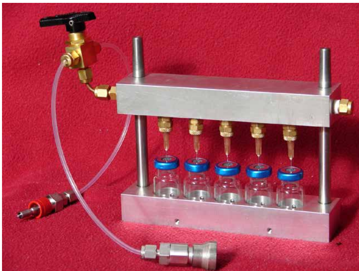
Figure 8.9: The Embrapa (Brazil) system for transferring samples from collection canister to 20 ml vials.
