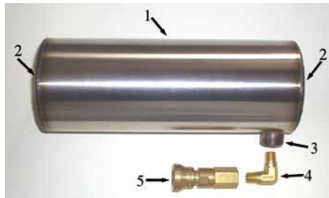
Figure 5.4: A 0.8 L stainless steel collection vessel used at the Department of Environment and Primary Industries, Victoria, Australia.
