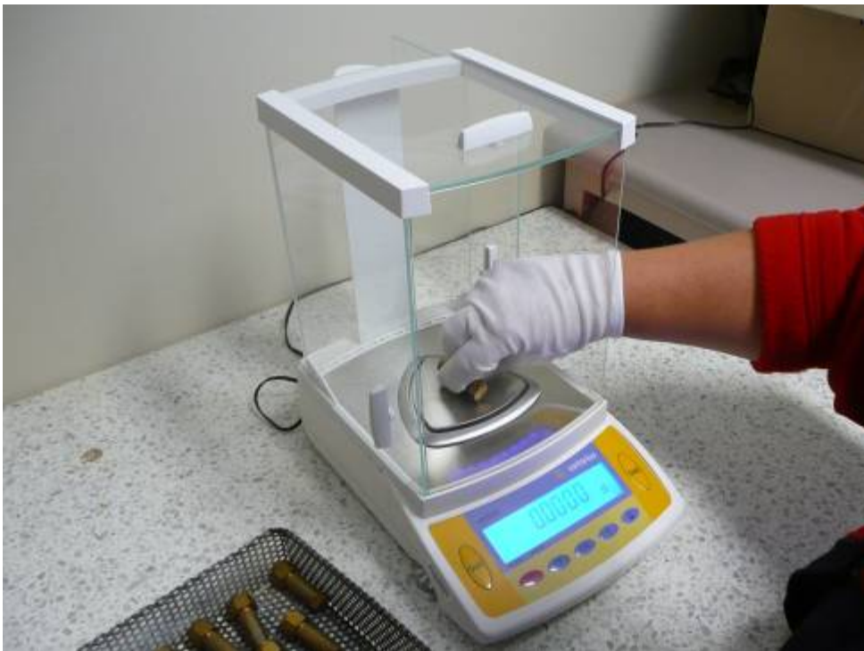
Figure 4.4: A Sartorius CP224S electronic balance as used to weigh permeation tubes at Department of Environment and Primary Industries, Ellinbank, Victoria, Australia.
