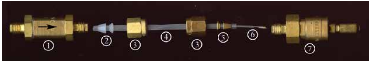
Figure 5.3: Air filter, flow restricting capillary tube and quick connect stem assembly used at the Department of Environment and Primary Industries, Victoria, Australia.
