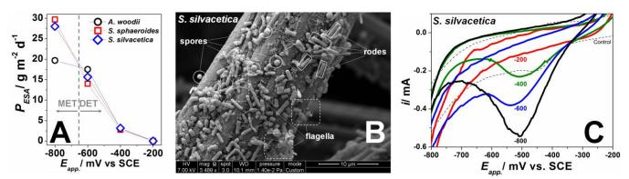
**Fig. 1.** A) P<sub>ESA</sub> vs. E<sub>app</sub>. during CA calculated according to Patil et al., 2015 (*Biotech. Adv.*). B) SEM picture of an electrode fiber cover by *S. silvacetica* cells. C) CVs at different E<sub>app</sub>. during CA.
