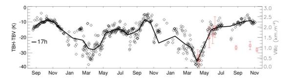
Figure 4: Evolution of the ELBARA Hpol-Vpol measurements from August 2011 to November 2013. Pics in Oct-Nov can't be explained with vegetation water content measurements (red symbols, right axis).
