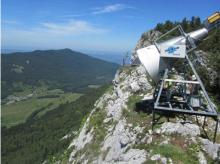
Figure 1: Design of the ELBARA experiment in the Vercors site. The radiometer is located at 1585 m looking at the studied area located at about 1000 m of altitude.
