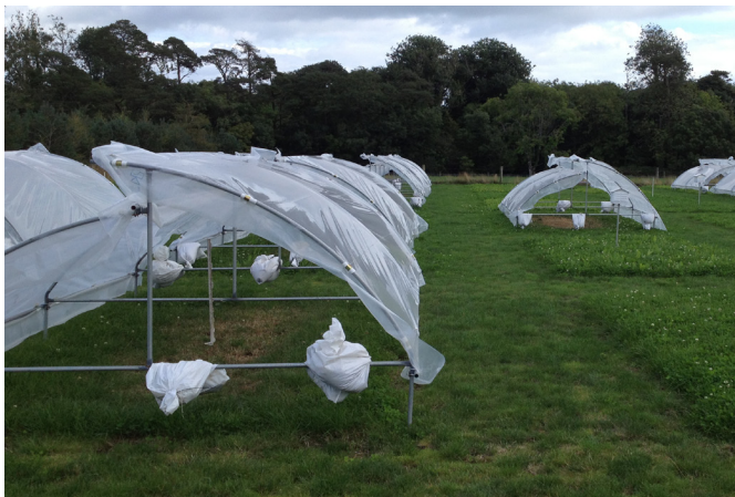
Figure 1. Series of 32 shelters used to exclude rain for ten weeks in a drought simulation at Teagasc (Ireland), and Agroscope (Switzerland). The 5m x 3m plots contain different species in monocultures, two-species and four-species plant communities.
