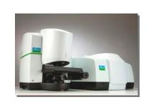
The system uses a rapid-scan Near and Mid/R spectrometer with a conventional FT-IR microscope. The custom-designed MCT linear detector array has 16 elements. Images are built up by stepping the sample stage. Stepping is synchronised with the interferometer scan, occurring as the scan direction is reversed, with the interferometer scanning continuous). This generates images at rates of up to 170 pixel/siscond. The image size is limited only by memory considerations.
