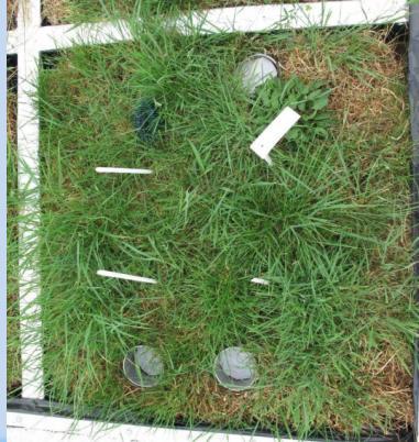
Soil respiration was measured with a Licor 6400 provided with soil chamber
