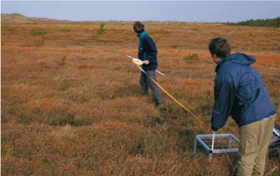
Figure 4.4: Data is sampled in a pinpoint frame supplied with data from a surrounding five metre circle.
