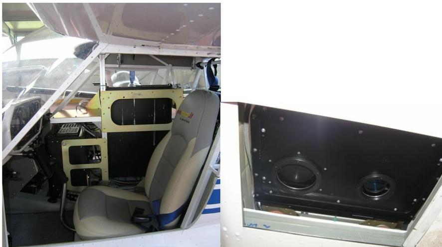
Figure 7: HYPER SIM.GA and UNIFI FOLDER installation and bottom view of optics
