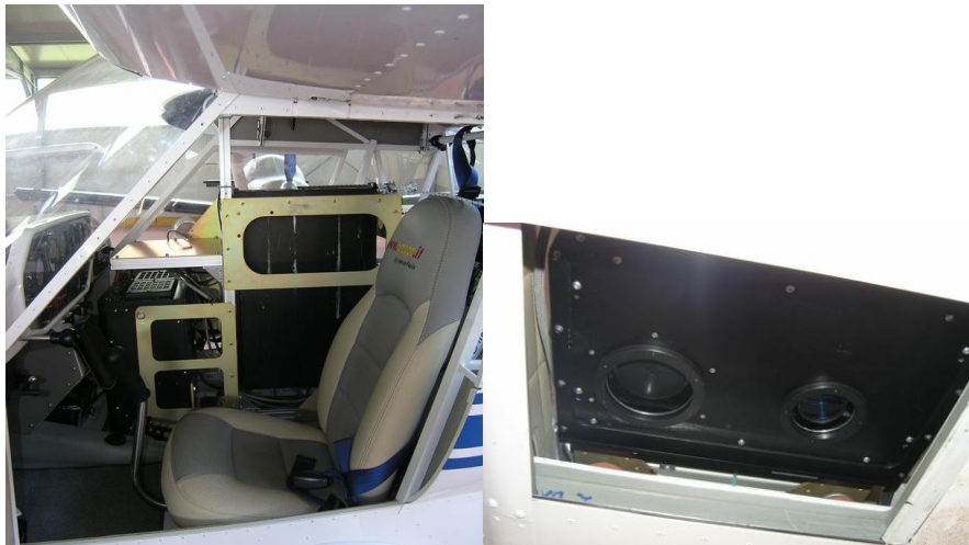
Figure 7: HYPER SIM.GA and UNIFI FOLDER installation and bottom view of optics
