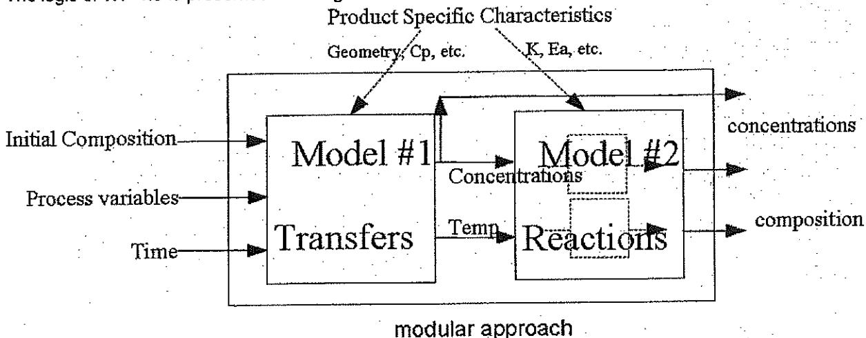
To model the process influence on antioxydative characteristics of food compounds, a modular approach is preferred. Two different categories of models will be designed:
