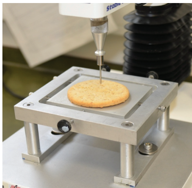
Figure 1. Biscuit assessment methods: Texture (2mm rod penetrometry).
