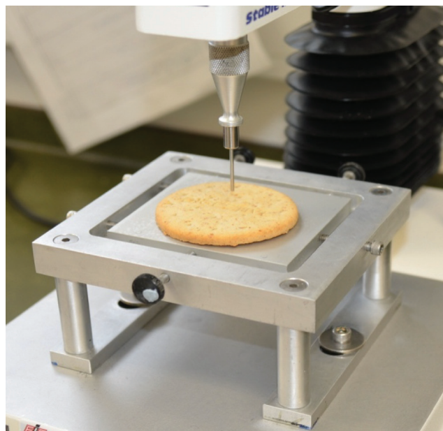
Figure 1. Biscuit assessment methods: Texture (2mm rod penetrometry).
