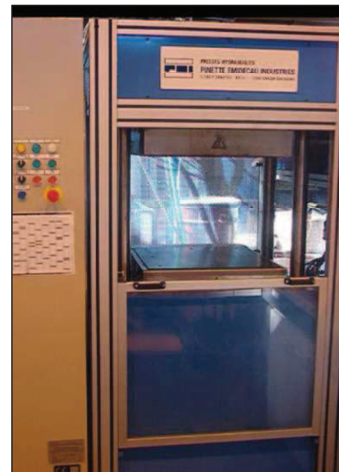
MAPA 50 heated hydraulic press (laboratory equipment)
