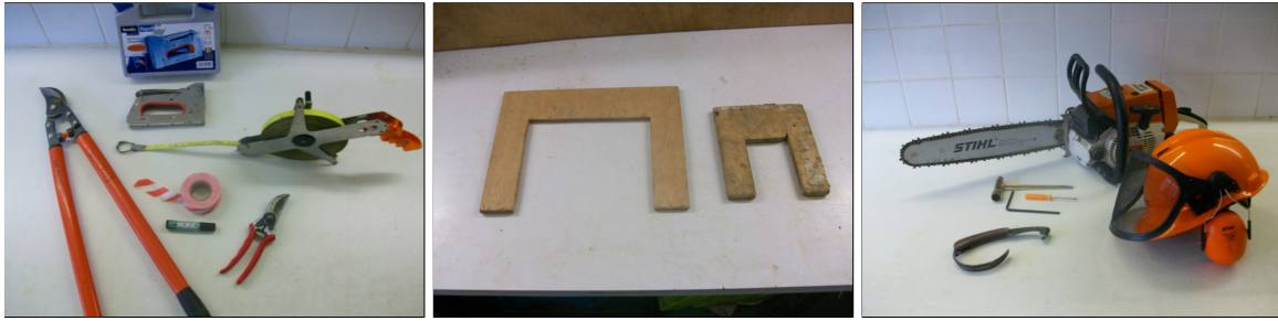
PHOTO 3.13 – Field equipment. Left, equipment for cutting and labeling aliquots; middle, typical gauges for cutting branches; right, power saw and safety equipment (photo: A. Genet).
