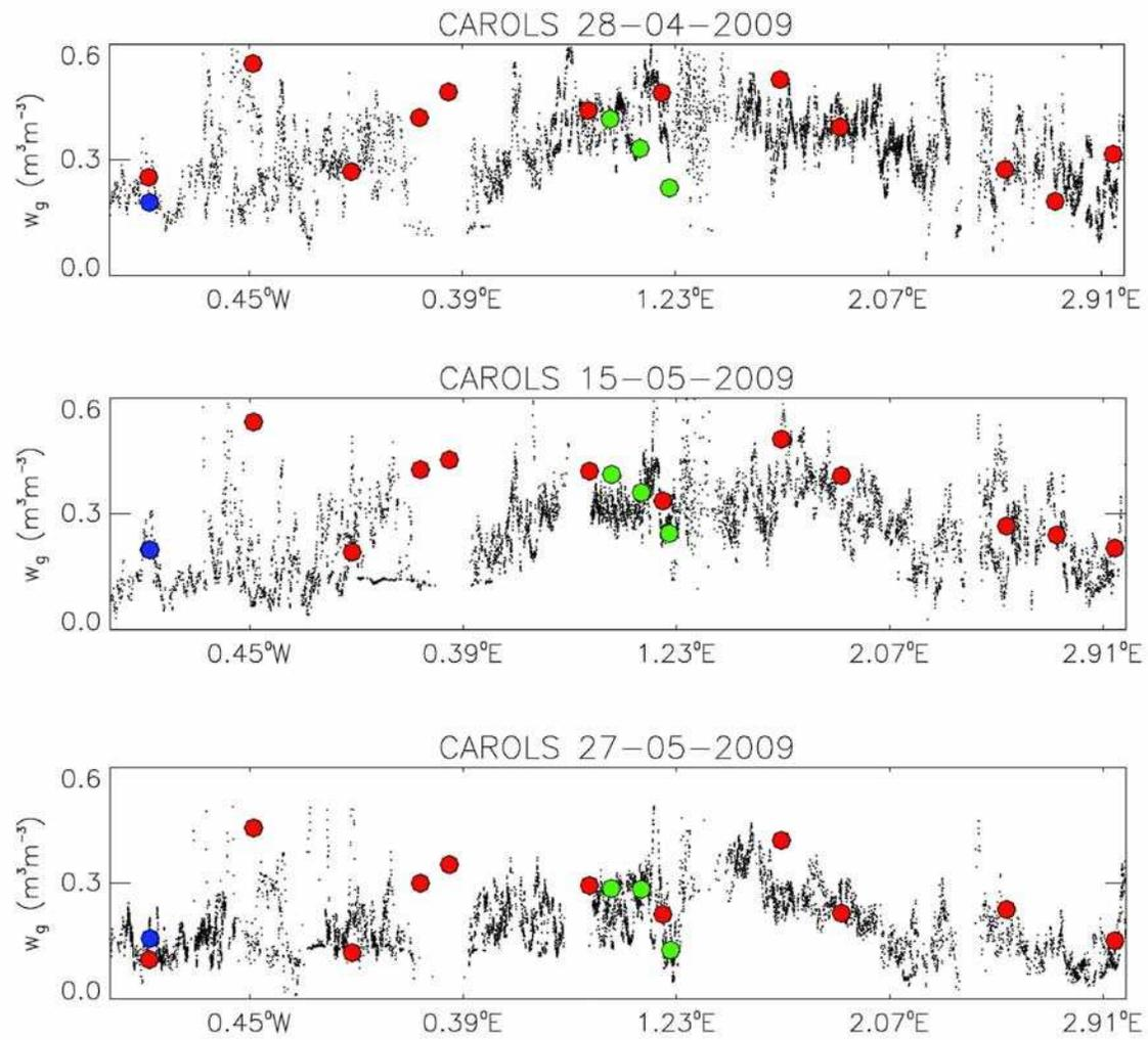
Figure 6. SSM retrievals ( $w_g$ ) based on the CAROLS TB in 2009, along the SMOSMANIA transect (small black dots) and the in situ SSM observations of the SMOSMANIA stations (red dots), from left to right the Le Mona, Lahage, Bérat sites (green dots), and additional observations in the Les Landes forest, by INRA/EPHYSE (blue dot).
