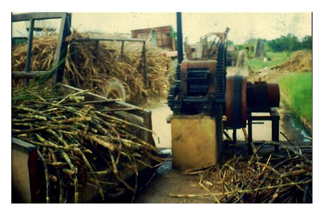
Figure 7: Sugarcane roller juicer at the SFC, Trinidad
