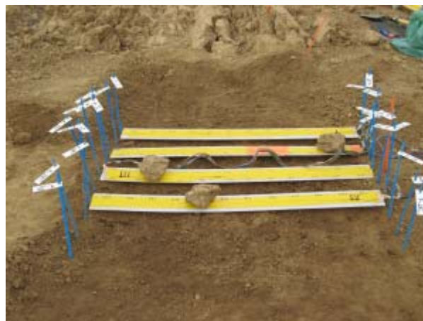
Figure 16: specific electrodes used for the characterisation of the soil structure at short scale. -a- plastic pan with electric electrodes spaced 10 cm apart. -b- Two plastic pans of 12 electrodes for a 24 Wenner array. -c- Four plastic pans of 12 electrodes for a 48 square array.
