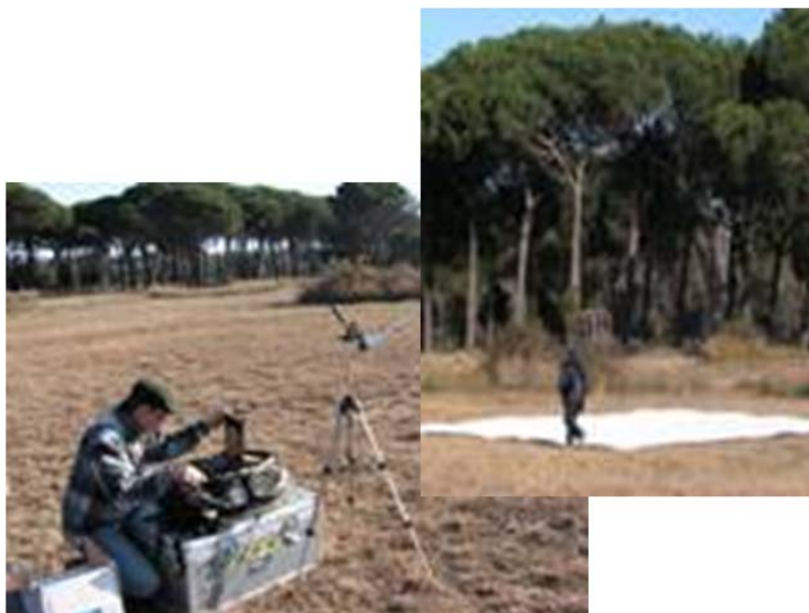
Figure 28 : Ground measurements for vicarious calibration.
