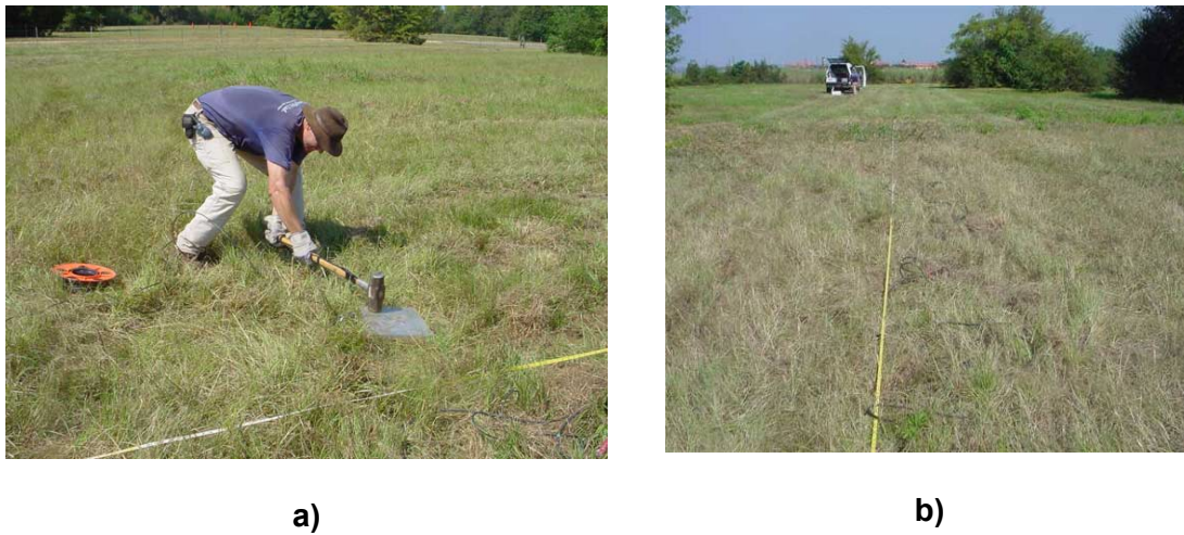
Figure 14: a) Impulse seismic source photography, b) linear profile of seismic sensors photography.
