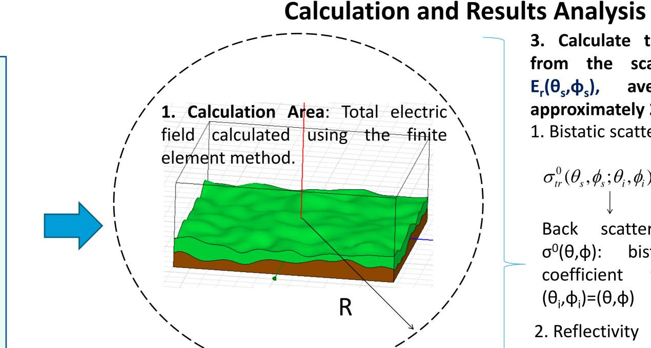
2. Near-to-Far Field transformation: The scattered electric field is calculated in the far-field region, at a distance R from the surface,  $E_r(\theta_s, \phi_s)$ .
