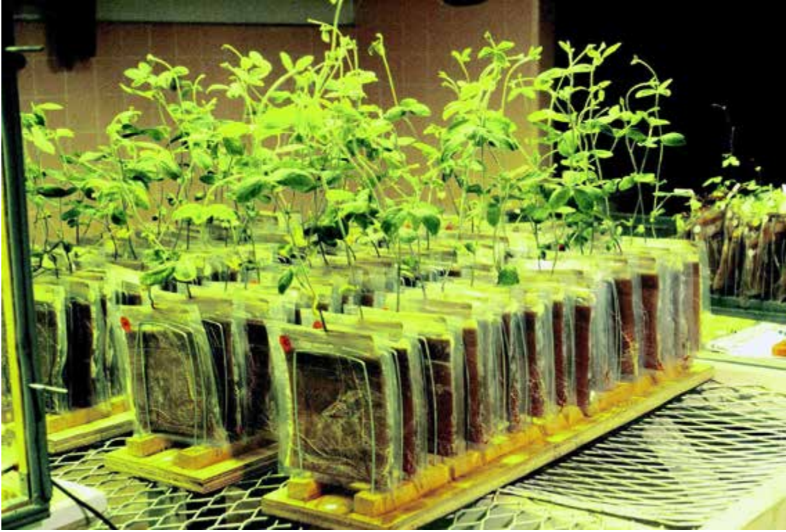
Fig. 2. Split-root growth assemblies arranged in home made racks - from wood and Al wire
