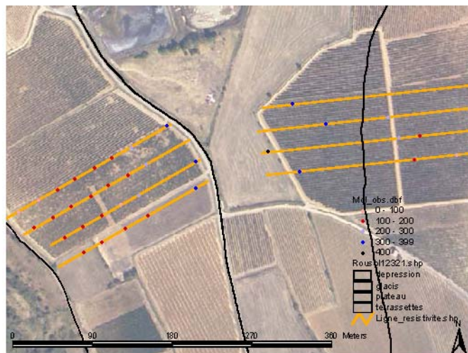
Figure 51: Position of boreholes (dots), MASW and ERT sections (yellow lines)
