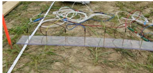
Figure 5: Focus on the system of electrodes used for the ERT measurement
