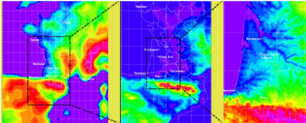
**Figure 1.** The three nested atmospheric simulation domains. From the left to the right the horizontal resolution is 32, 8 and 2 km, respectively. The largest domain covers part of Western Europe, the intermediate one includes parts of France and Northern Spain and the smallest one focusses on the Aquitaine region. The colours are indicative of the topography.
