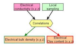
Figure 3: Estimation of bulk density and clay content from electrical conductivity
