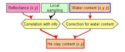
Figure 7: Estimation of clay content from reflectance
