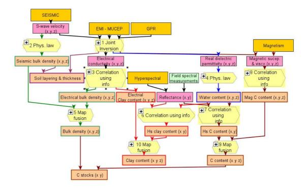
Figure 11: Scheme of the general processing workflow
