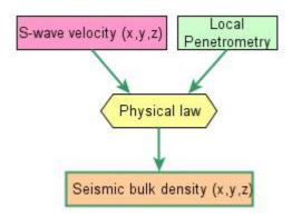
Figure 5: Estimation of bulk density from S-wave velocity
