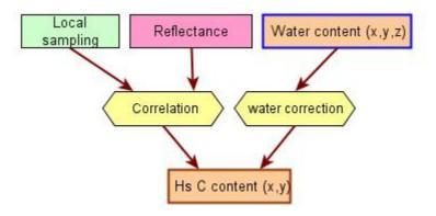
Figure 6: Estimation of carbon content from reflectance
