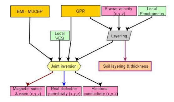
Figure 1: General scheme of the joint inversion
