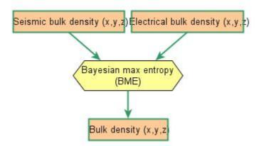
Figure 8: Fusion mapping of bulk density
