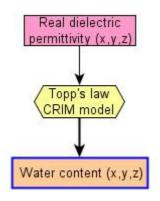
Figure 2: Estimation of water content from dielectric permittivity
