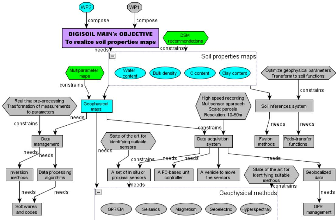
Figure 11 : Schematic functional analysis of the Digisoil production: deliverable D2.1 tasks are highlighted
