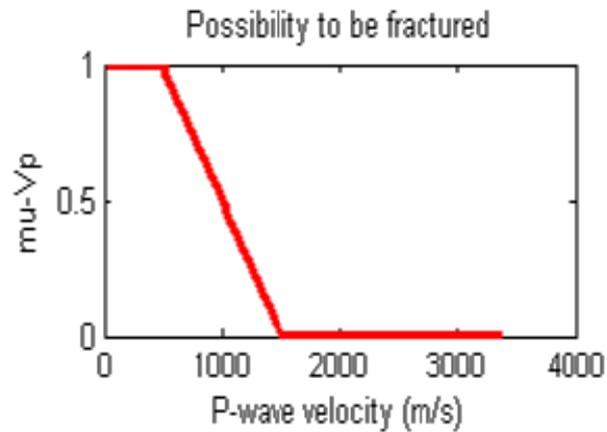
Figure 3 : belonging function used in fuzzy logic method. This function gives the possibility that a material is fissured depending on the value of  $V_p$ .
