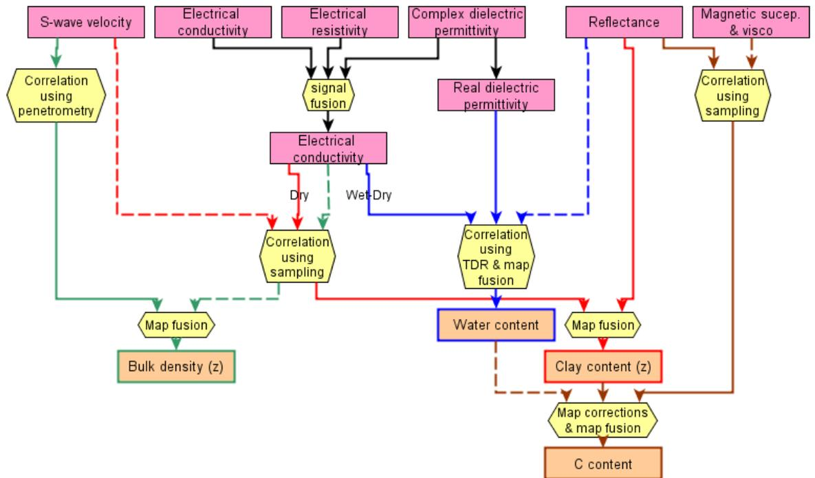
Figure 10 : data assimilation from geophysical parameters to soil properties
