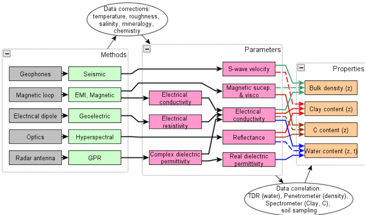
Figure 1 : diagram showing the different paths for going from sensors to soil properties.
