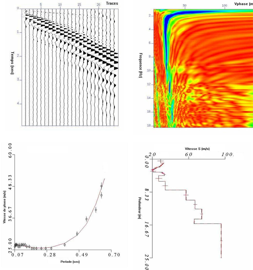
Figure 9 :a-Example of short record with obvious low velocity Rayleigh wave (b)- Phase velocity plot obtained by interception time ray parameter transform c- Experimental and theoretical phase velocity fitting by linear inversion d-Depth variation of shear velocity.
