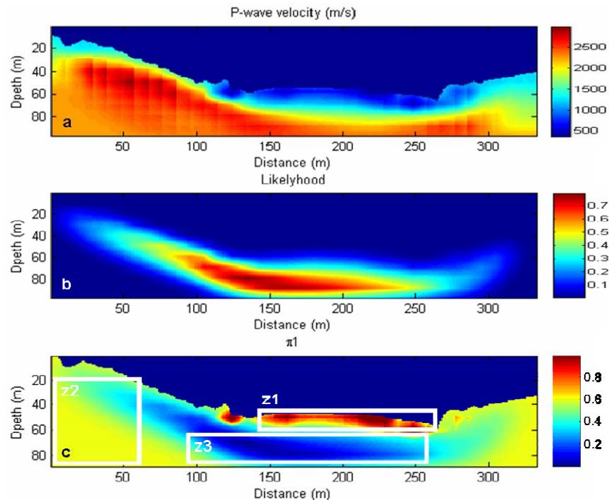
Figure 4 : Example of fuzzy logic rule for translating P-wave velocity ( $V_p$ ) and its likelihood function ( $LV_p$ ) into a map indicating the possibility ( $p_1$ ) that the rocks are fissured (Grandjean et al., 2007).
