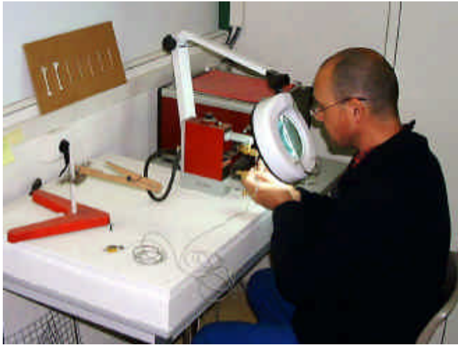
Figure 2-6: To weld thermocouple sensors
