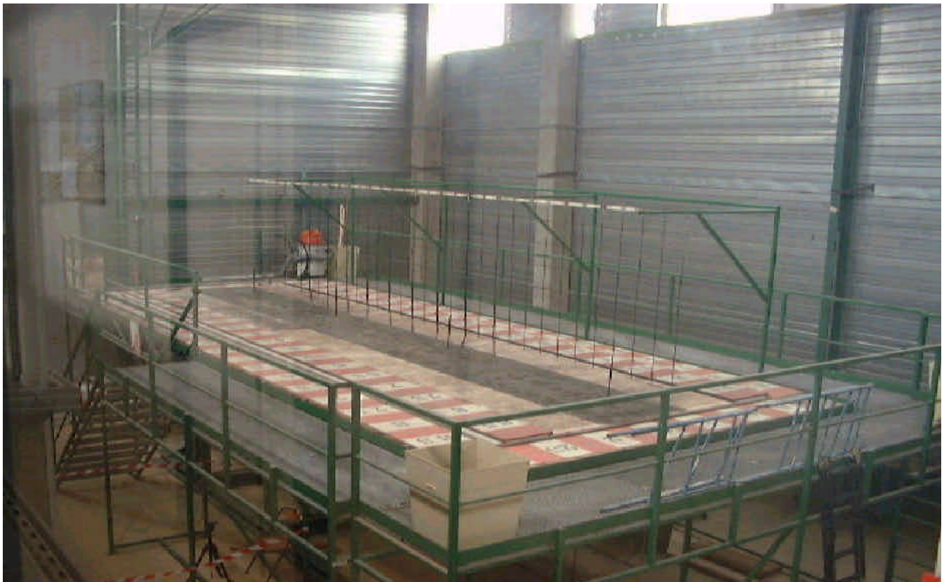
Figure 4-1: General view of the experimental bench for moving fire DESIRE
