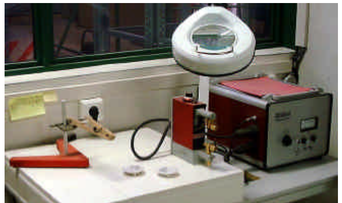
Figure 2-5: The welding machine Soudax SD 100
