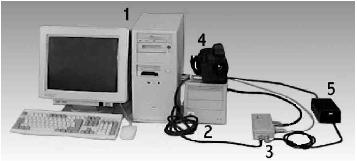
Figure 7-2: ThermaCAM® Researcher HS - ThermaCAM® SC parallel interface system
