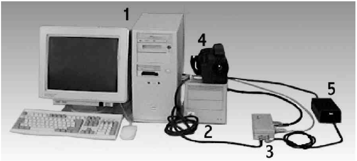
Figure 7-2: ThermoCAM® Researcher HS - ThermoCAM® SC parallel interface system
