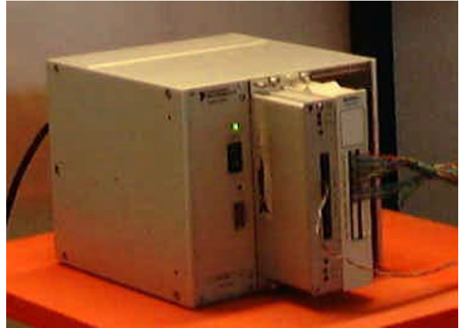
Figure 5-1: SCXI100 chassis, SCXI1321 and 1303 connectors
