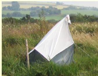
Emergence trap (based on Malaise trap model)
