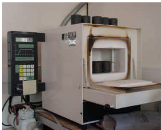
Figure 3-2: The furnace and its electronic controller and the five containers
